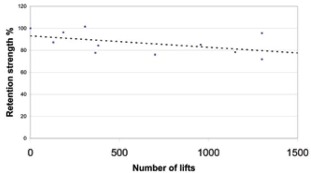
Retention strength of sling versus number of lifts.
