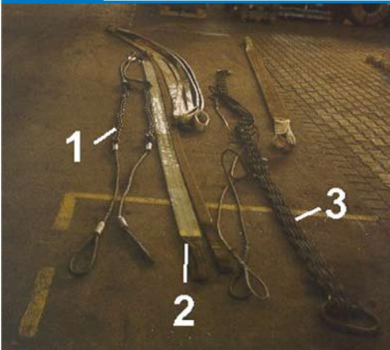
Various kinds of slinging equipment are used for handling sheet metal coils: (1) wire rope sling combined with central chain sling; (2) webbing sling made from polyester with solid polyurethane coating; and (3) chain sling.<sup>1</sup>
