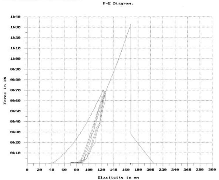
Typical elongation behavior of a 20-ton (SF 7), 3.8-m sling under load.
