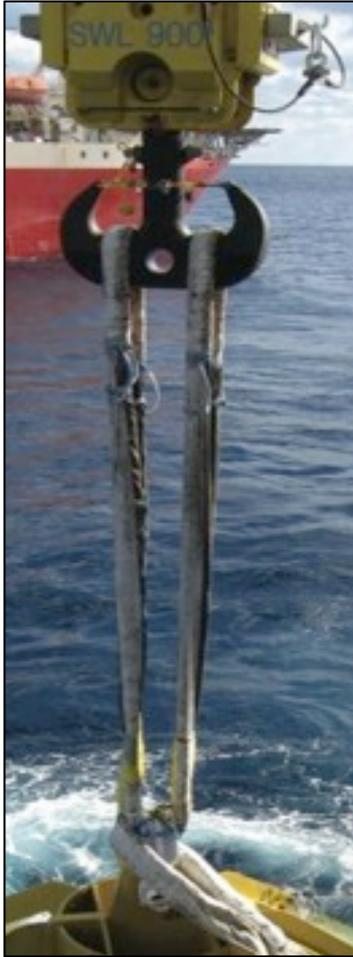
handling low weight slings instead of the burdensome steel sling. Also lifting tower sections for wind turbines find a useful application in HMPE slings, as they do not damage the coating of the piles.
