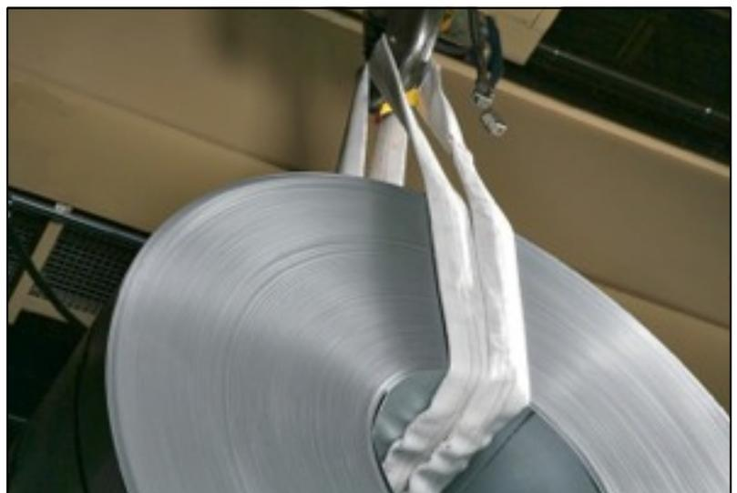
For lifting of steel coils at the Corus steelworks, Technotex in Holland together with DSM Dyneema®
